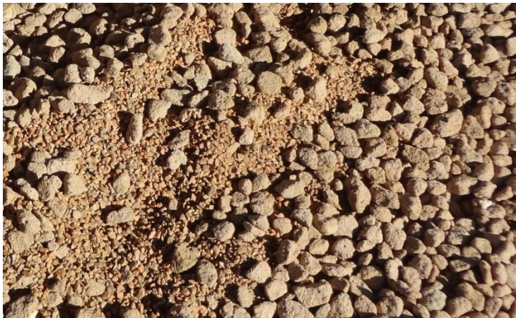
Figure V.7. The filter material Polonite, used for sorption of dissolved phosphorus in agricultural stream water. Photo: K. Tonderski, POMinnO Sp.zo.o.
