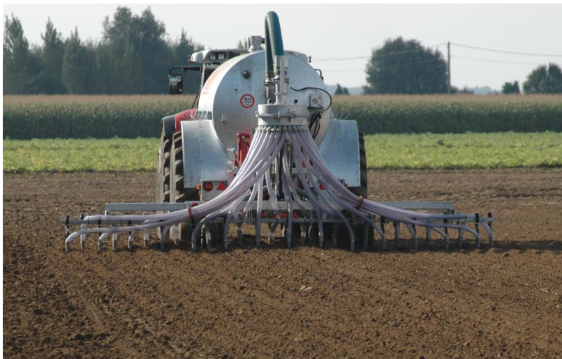
Figure IV.27. Application of manure with an applicator for deep injection. Photo: Werktuigendagen.
