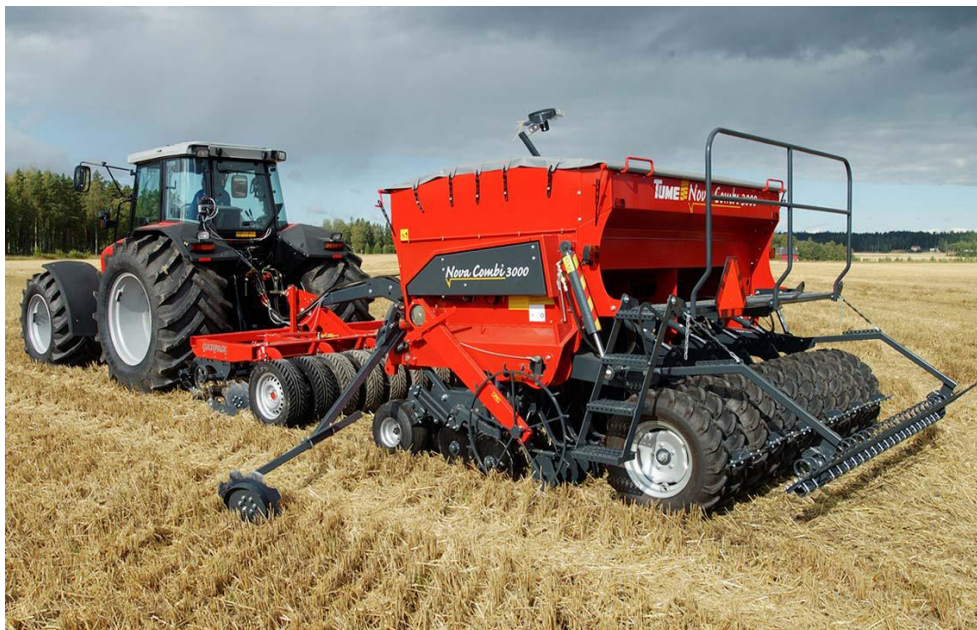
Figure IV.23. Equipment for simultaneous sowing of seeds and fertilisers (combi-drilling). Source: Nilsson [2005].
