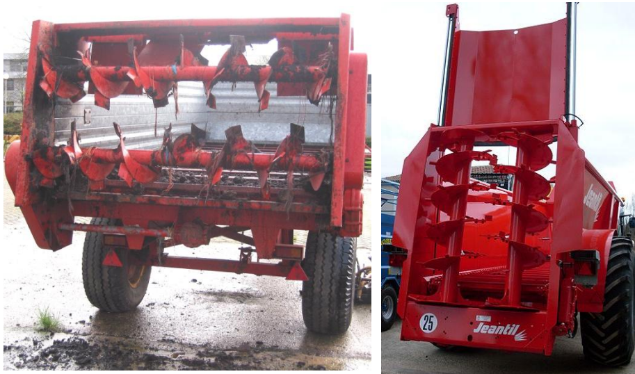
Figure IV.25. Manure spreaders for rear and side spreading. Photos: LORIMOR [2000].
