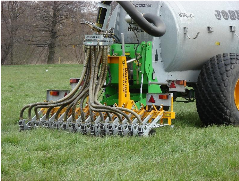
Figure IV.26. Liquid manure applicator for shallow injection of liquid manure. Photo: P. Nawalany.
