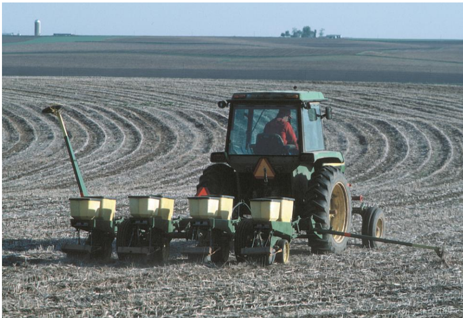
Figure IV.31. Equipment for direct drilling. Photo: Gene Alexander.
